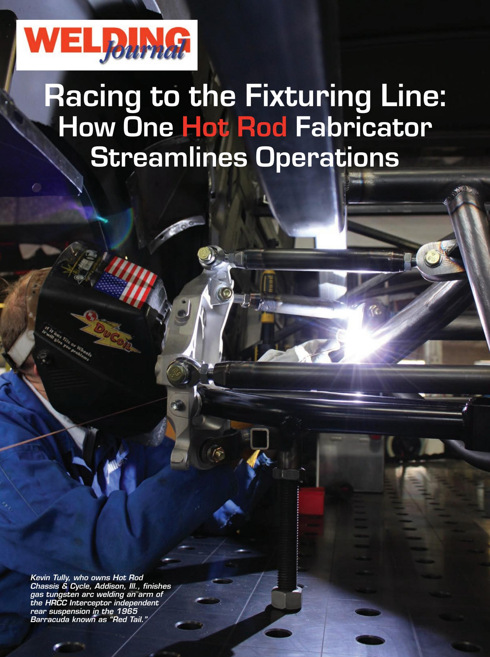
*Kevin Tully, who owns Hot Rod Chassis & Cycle, Addison, Ill., finishes gas tungsten arc welding an arm of the HRCC Interceptor independent rear suspension in the 1965 Barracuda known as "Red Tail."*
