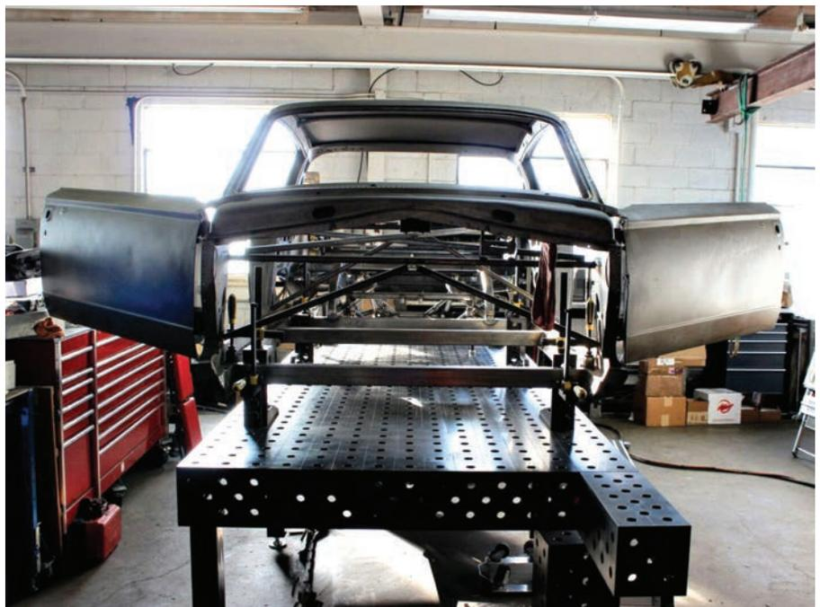
*Fig. 2 — Temporary cross members and fixturing are seen on this vehicle.*
