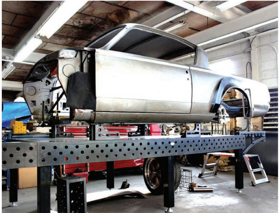
*Fig. 1 — A '65 Plymouth Barracuda is shown fixtured and getting its new frame installed.*
